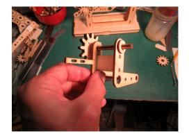
Slide the shaft with the gear into the position shown and glue the remaining thicker washer on the back side. Again, apply some pressure with your fingers to remove any slop in the assembly.
