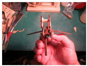
Apply even pressure with your fingers, pushing the leg up against the profile and hold it for a minute or two. The leg should be parallel to the profile figures as shown on the right photo. Rotate the leg a bit just to make sure it hasn't been glued to the profile.
