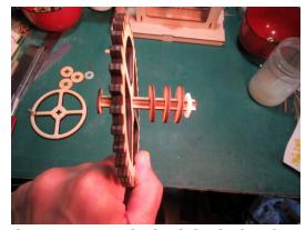
Locate the parts shown on the left photo. All washers are 3mm thick. Slide shaft 4 through the large 36-tooth gear and then stack three of the large washers behind it and the nylon shoulder washer.
