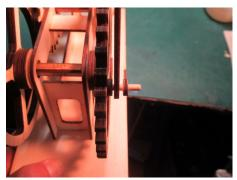
On the front side, slide the link up against big gear's face and the stepped shaft's face. Slide a small washer onto the dowel pin of the big gear and another small wooden cross washer on the stepped shaft. Apply a small amount of glue to the outside of the washers and then slide them out a bit, leaving a small gap. Repeat behind. The lower part of the kit is now complete. It's time to work in the mechanism.
