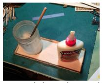
Glue on the two shorter sides first then follow it up with the two longer sides. Don't forget to put glue in the corner tabs as well. Place some weights inside the base while it dries. This will remove any warp.
