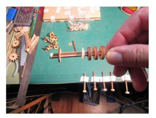
Slide the thin, 1/16" thick washer, 5/8" outside diameter down the shaft and using a toothpick apply a small bead of glue around the end of the shaft. Run up the shaft the same stack of washers used previously for the axle caps. Make sure the nylon washer is going up against the thin washer.
