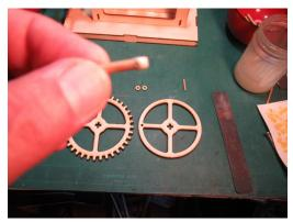
Locate the large 36-tooth gear and the wheel, the two little dowels and the two small washers 1/8" inside diameter and 3/8" outside diameter. Apply glue to the bottom of the dowel and place it in the small hole of the wheel.
