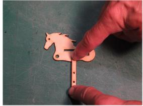
Flip over the Pegasus profile that has the extension on it so that the engraving is on the back side. Glue this doubler onto the extension. Make sure to align the holes. This part has a nagging tendency to slip out of alignment so take extra care while holding this down and that the edges stay aligned.
