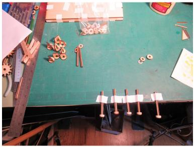
Follow this procedure for five of the seven shafts. Here they are drying, all axle caps are perpendicular the their respective shafts.
