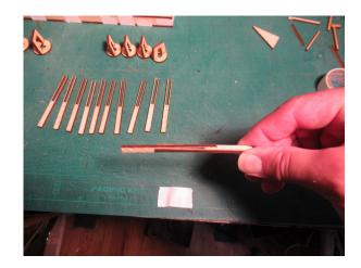
Slide the two half shafts together as shown. Make sure to slide the shafts all the way to the end and make sure the ends are aligned with each other. No glue should come out. If it does, wipe it off with the moistened brush and make sure to use less glue on the next one.
