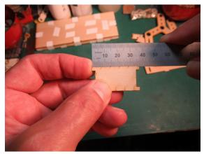
Time to assemble the frame. Gather the parts shown on the left photo. Make sure the shaft designations (the small crosses) are on the outside. Also, check that the spacers are about 35 mm long.
