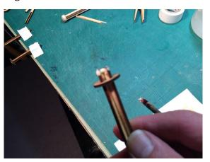
Here's how it should look. With shaft 4. you are going to glue on a thin (1/16") thick washer, 3/4" outside diameter) onto the end of the shaft using a similar method to what you did before. Slide the washer down the shaft and apply glue using a toothpick.
