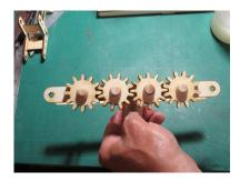
Put glue around the back side of the shaft, then place the washer over the shaft. Apply some pressure with your fingers as shown on the middle photo. Make sure there are no gaps or play in the shaft. Hold that pressure for a minute or so and then carefully place the ladder down so as to not allow any shifting in the parts as they dry.
