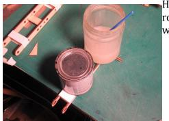
Hang the lower link off the side of the table so that the rounded end doesn't prevent it from laying flat. Place some weight on it while it dries, as shown here.
