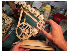
GENTLY ROTATE ANY AREAS THAT OFFER RESISTANCE. A GENTLE BACK AND FORTH MOTION WORKS BEST. AFTER SEVERAL ROTATIONS THE MECHANISM WILL START TO FREE UP AND BECOME VERY SMOOTH. MAKE SURE TO ROTATE THE HANDLE IN BOTH DIRECTIONS.
