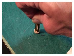
Glue axle caps onto the ends of shafts 1-3. If you have trouble getting the axle cap on, you can try tapping it on the table top. Remove any excess glue with the moistened brush.
