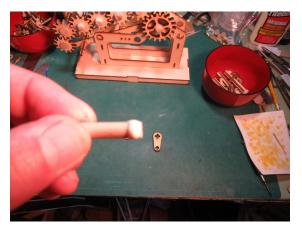
Assemble the handle by placing a generous bead of glue on the flat end of the ¼" dowel.
