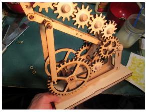
Slide a small wooden washer (½" outside diameter and cross center) onto the lower link's stepped shaft. Then slide the wooden links onto their respective shafts as shown in the photo on the right. The side with the smaller hole goes into the big gear on one side and the big wheel on the other side.
