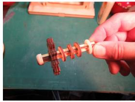
Time to put in shaft 3. Gather the parts shown here. All those wooden washers are 3mm (1/8") thick and 34" outside diameter. Slide shaft 3 through the 12-tooth gear followed by three wooden washers (all 3mm thick) and then the nylon shoulder washer.
