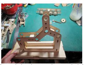
You are now going to attach the ladder to the frame. Gather the parts shown at the left. Place two of the nylon shoulder washers at the top of the frame as shown on the right (front and back).
