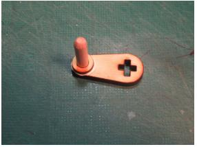
Place the dowel into the handle base. Make sure it's all the way at the bottom. Tap it if necessary. Glue will come out the top. Now slide the washer ( $\frac{1}{2}$ " outside diameter and  $\frac{1}{4}$ " id) down the dowel. The glue at the bottom will be more than enough. Now wipe off excess with moistened brush.
