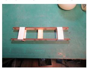
Glue the top piece on. If the warp is severe, apply tape to the two ends and lay flat while drying. Place some weights on it while it drys. Make sure the tape is longer enough to go all around.
