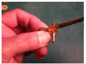
Take one of the shafts and slide one of the cams onto it. The face that is shown at the left should be in the center of the shaft. Now apply glue to this side of the cam and all around the shaft interface. Then slide the other cam onto the shaft. Remove any excess glue with the moistened brush. Also make sure that the cam is approximately in the center of the shaft and that the two half shaft pieces stay aligned at the ends.
