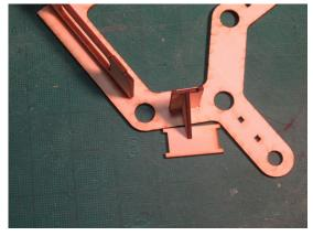
Start by gluing in the longer side piece. Make sure the tab is pointing down. Use the square to ensure perpendicularity. Glue in the other side and the spacers, always using the square to ensure
