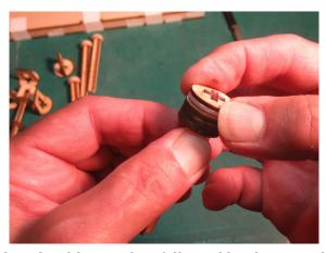
Again slide the stack of washers, the larger nylon shoulder washer followed by three washers, 3mm thick and 3/4" outside diameter. Slide the thin washer to the end and wipe off any extra glue with the brush. Again apply downward force on the washer while applying upward force on the stack of washers to ensure perpendicularity. You can allow a tiny amount of the shaft to protrude and sand flat when fully dried.
