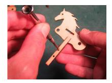
As you did once before with the gears, run one of the 2-56 screws into the hind leg and the front leg as well as through the two holes in the extension piece of the Pegasus figure. Creating the threads in these four holes makes final assembly much easier. Remove the screw when you're done.
