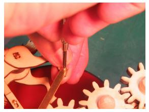
Screw this side of the link into the gear as shown. **These screws do not get tightened.** Leave a gap (1/16") between the head of the screw and the washers. Keep it loosey goosey. Now place the shorter brass screw through the other hole of the brass link and place one washer under that. Rotate the link until it aligns with the hole in the hind leg. Screw it down, remember keep it loose.
