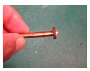
Glue together the two shorter half shafts (2 inches long) as you have done previously and then glue to one end, the small 3/8" outside diameter washer with the cross in the middle. Place this washer about 1/8" from the end of the shaft. Set aside to dry.
