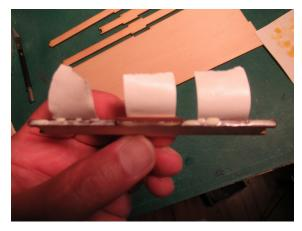
While the jigs dry, assemble the base. Start by gluing a short side on first. Apply tape to the outside of the piece and using the brush apply glue as shown. The tab gets the glue on the inside.
