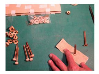
Here are all seven shafts drying. Only after a very long drying time, several hours, you can sand the two shafts with the thin washers on them. Flip them upside down and either using sandpaper or an Emory board, sand the face flat. This is an optional step done mainly for aesthetics. Be gentle with this part and don't knock off the washer while sanding, a few strokes is all it needs.
