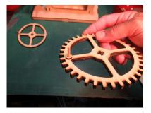
If some glue comes up that's fine, now place the small washer on top. Do the same with the gear. Remove any excess glue with the brush.
