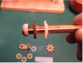
Locate the parts shown here, that's shaft 1. All those wooden washers are 3mm thick. Slide on a wooden washer followed by a nylon shoulder washer.
