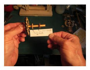
Gather the parts shown here along with shaft 2. Three of these wooden washers are 3mm thick,  $\frac{3}{4}$ " outside diameter, and one washer is  $\frac{1}{16}$ " thick. Slide shaft 2 through the 18-tooth gear and then place a thin,  $\frac{1}{16}$ " thick, washer followed by a 3mm thick washer behind the gear.
