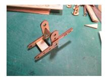
Gather the parts shown at the left. Note these spacers are the same type used on the frame, about 1.4 inches long or 35mm. Using the square, glue in spacers. Glue on top piece, note the doubler is on the outside.
