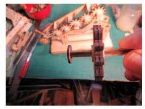
Slide the Pegasus stand in between the ladder as shown. Again place nylon shoulder washers on either side of the gear and pass the shaft through.
